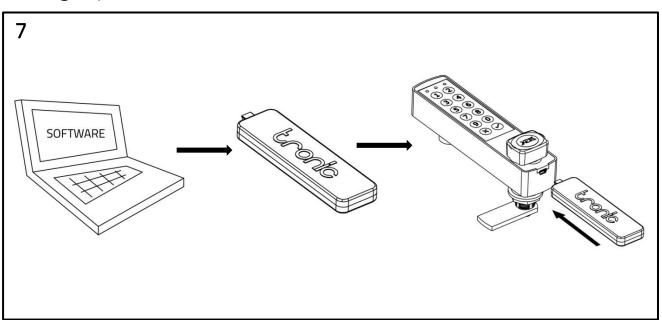
Load settings from the computer to the settings key (BLACK). Connect settings key to the lock.
