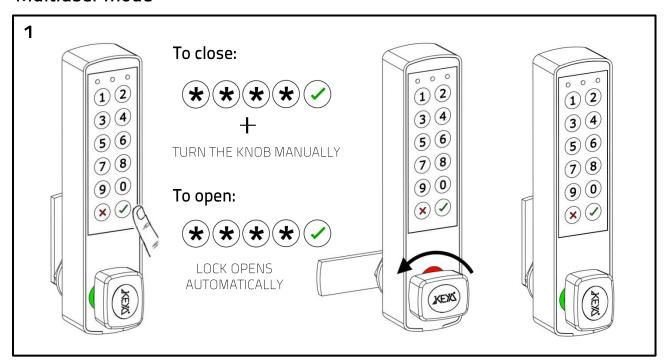
Open and close by 4-digit code. The code is deleted every time the lock is opened, being available for new user.
